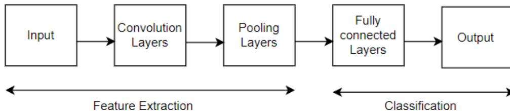
Fig 1: general architecture of cnn
